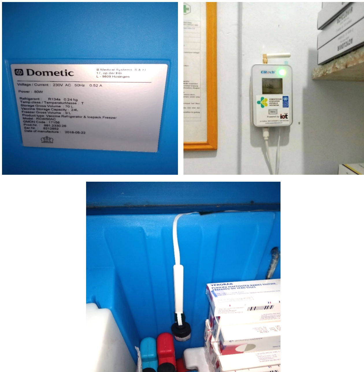
Figure 16. Temperature logger installation for vaccine storage 2-8°C
